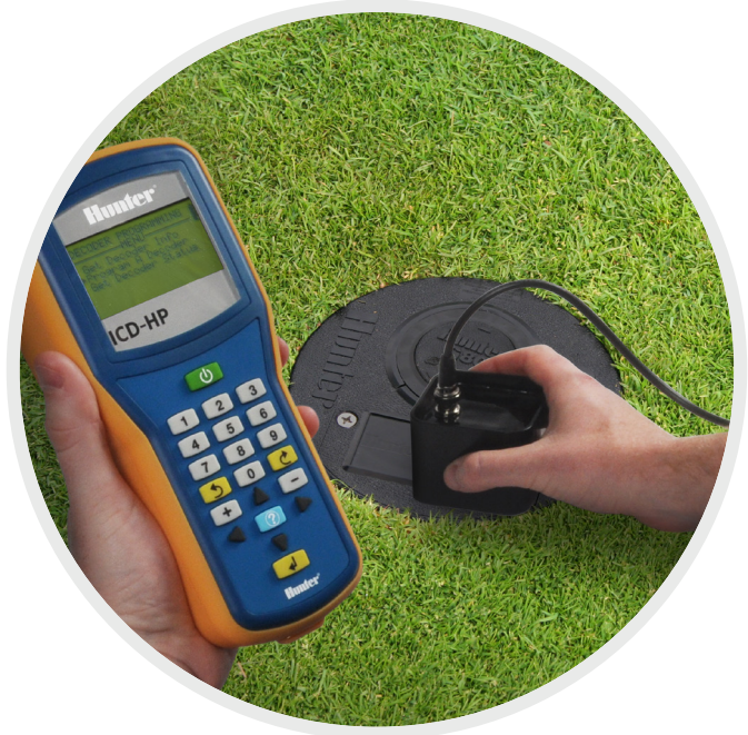
ICD-HP programming screen for a six-station two-way module
