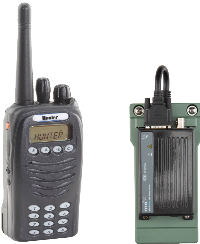
TRNR Maintenance Radio and PILOT-MOD-UHF Radio Module
