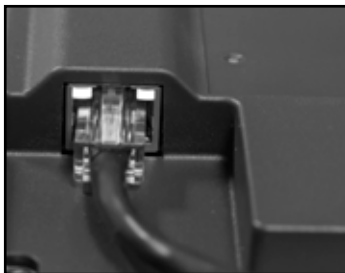
Network Lights (back of Com module)
